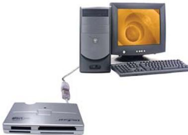
Connect your card reader to your PC (note: be sure that the card reader driver is installed) and insert the Compact FLASH card (we recommend 128 MB minimum) into the reader. To program your multimedia content on to the media card, open the file manager and copy the files to the card reader drive.
