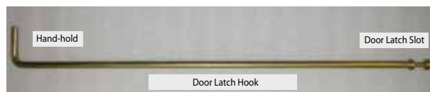
Figure 22b. Door buckle tool
