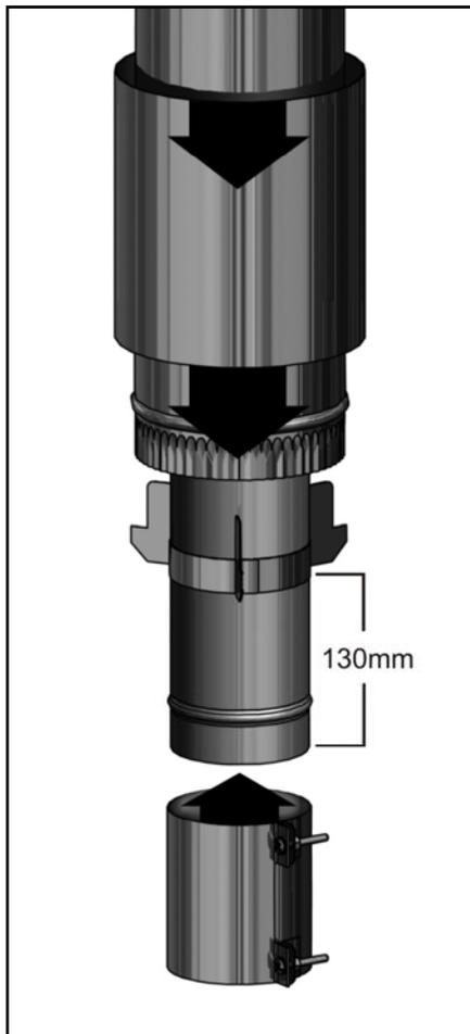
The bottom section is similar to the top assembly. The flue spacer bracket must be secured 130mm from the end of the 100mm flue, this will give clearance to slide the flue sleeve up the flue when installing the Fireplace. Once the installation is complete the 180mm flue sleeve can be slid down to cover and protect the lower assembly.
