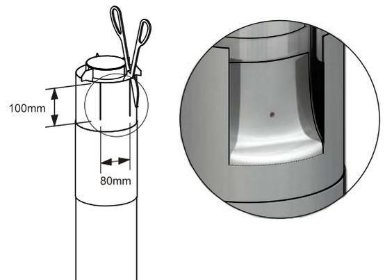
Fit cowl and drill trough the flap, flue and cowl stem. Using approximately a 1" stainless steel self tapping screw fix the cowl in place.
