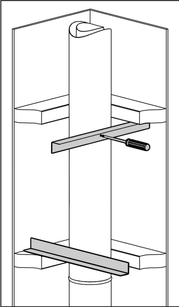
A length of Angle should be attached to the inside of the timber frame cavity to hold the flue in place. Once you have fixed the Angle to the inside of the cavity holes must be drilled to secure it to the flue. Screws or rivets can be inserted directly into the 150mm flue to hold it in place.
