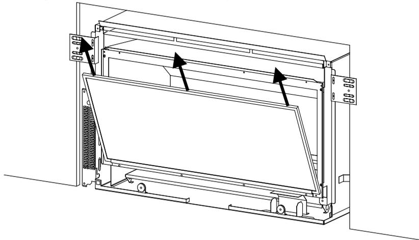
**Step 3:** Remove the top of the heater outer shell. Take out the screw from each side (as shown below), lift and pull the top of heater shell out towards yourself.
