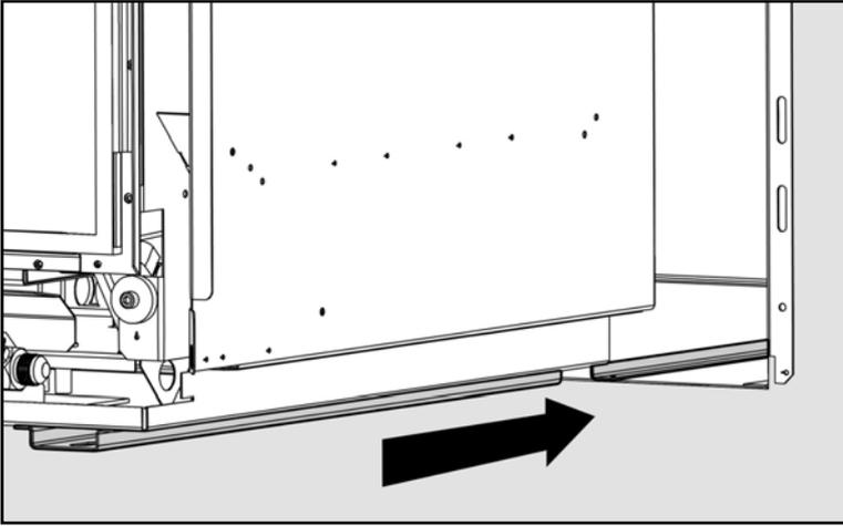
Attached to the base of the Outer Skin Kit are guide rails. The inside edge of these rails will line up with the outside edge of the two outer under base supports. When the parts are lined up, push the fire towards the back of the Outer Skin Kit until it cannot be pushed back any further. The front of the firebox should now be sitting flush with the OSK.
