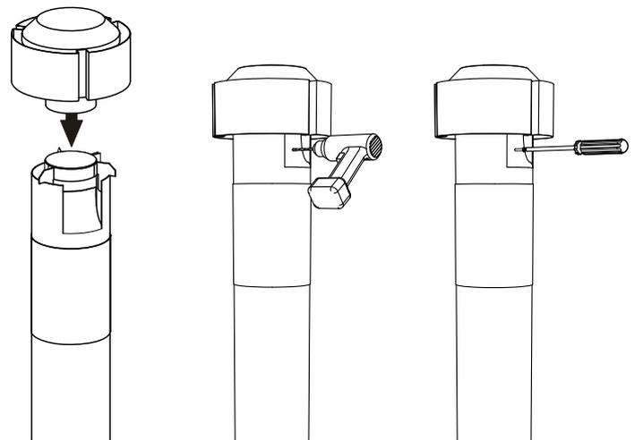
Slide the liner sleeve piece up under the cowl until it hits the flue spacer bracket. Around the bottom of the sleeve drill and rivet in three places.
