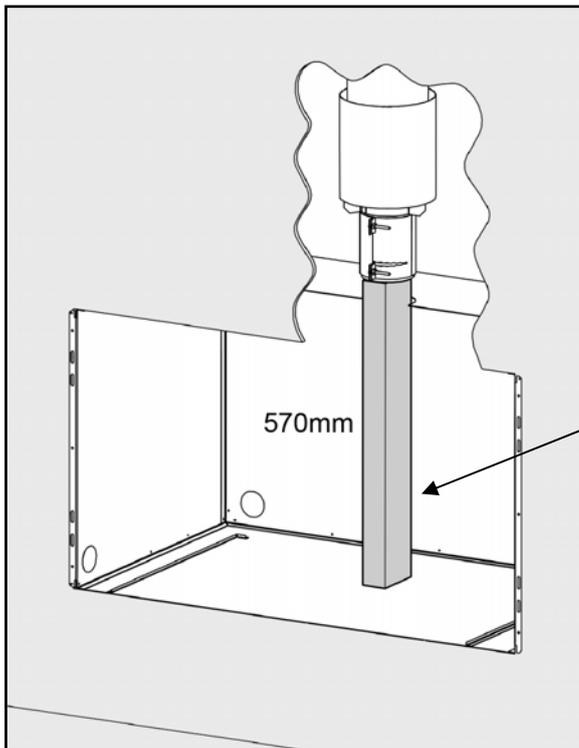
To make sure the flue is installed at the correct height, a piece of timber can be cut to 570mm and between the fire base level and the bottom of the flue. This will ensure the correct height for installation and support the flue assembly.
