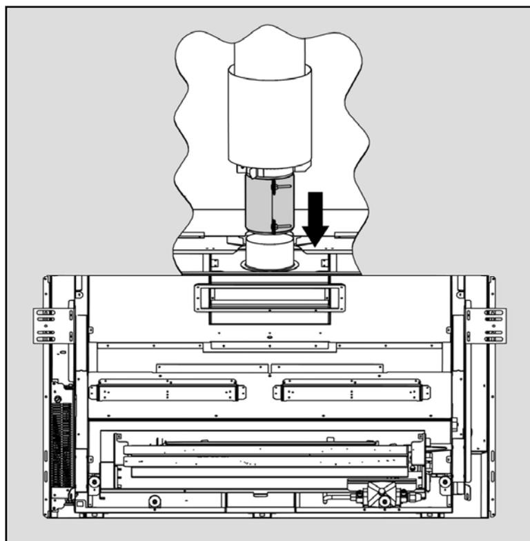
Once the gas fireplace has been inserted into the OSK and the firebox removed, the flue can be attached. To do this line up the 100mm flue with the flue outlet spigot then slide the clamping flue sleeve down onto the spigot.
