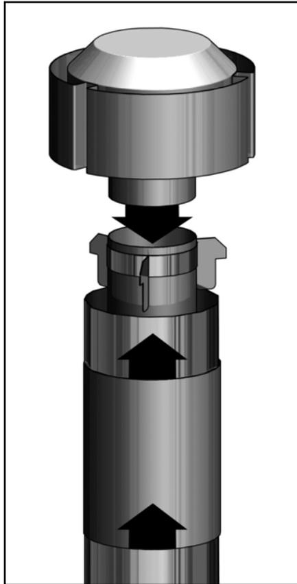
Secure the Flue spacer bracket to the top section of 100mm Flue and insert the cowl, this can be riveted or held in place with screws (see 12.1 Installing the Flue Terminal). Now slide the 150mm flue onto the bracket.
