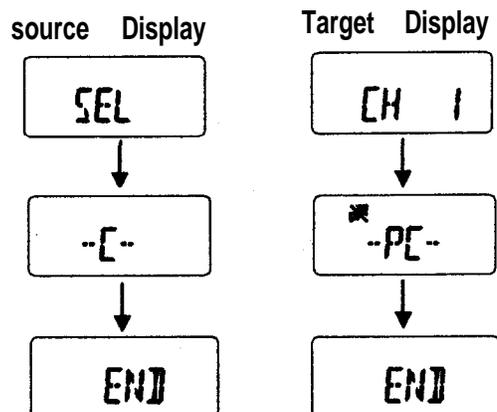
7. To done another target unit turn off the target unit, remove the CCRP cable from the target unit, connect the CCRP to another target unit, and switch the unit on.
