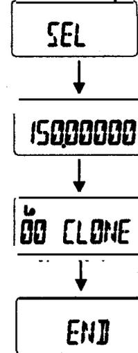
When cloning is successful, "END" will be shown on the displays. If "ERROR" is shown on the target's display, start the cloning process over. Make sure the batteries are fully charged and that the source and target units are in close proximity to each other.
