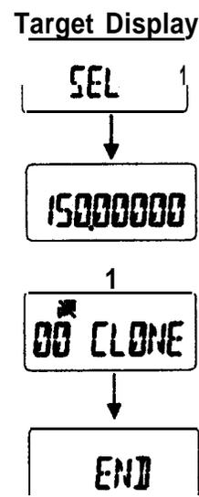
3. Press the [MONI] button to enter the wireless clone mode. A frequency will appear in the display. Adjust the channel select knob to adjust the frequency to the desired frequency to receive data on. Note: Pressing the [LAMP] button while turning the channel selector will change the frequency in 1 MHz steps.
