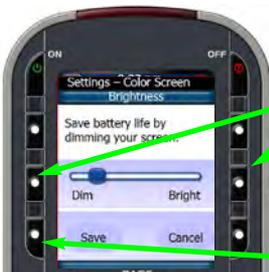
Use the DIM and BRIGHT buttons to adjust the lighting of the color screen.
