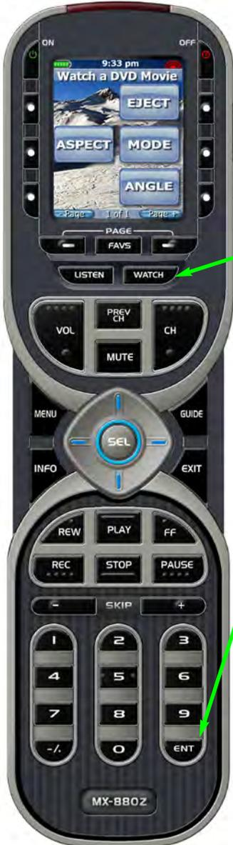
Simultaneously, press and hold both the WATCH and the ENTER buttons. When the SETUP screen appears, release the two buttons.
