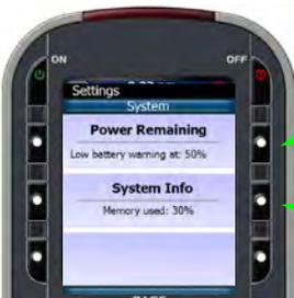
Select Power Remaining to check your power remaining or to set a new battery warning level.
