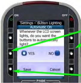
Use the YES and NO buttons to set the button back lighting to automatically turn on or not.
