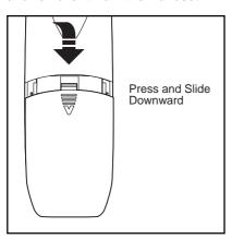
Install the BATTERY PACK, with the metal contacts facing down and aligned with the Handset contacts. Replace Handset battery cover.
