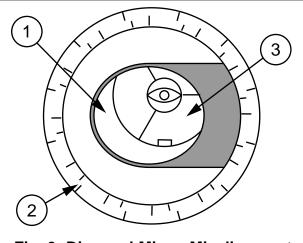
Fig. 9: Diagonal Mirror Misalignment
