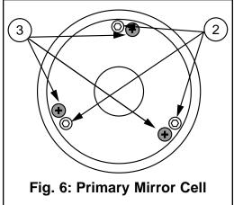
falls directly through the center of the focuser drawtube (17, Fig. 1). These mirror tilt adjustments are made with the diagonal assembly (Fig. 5) and the primary mirror cell (Fig. 6), and will be discussed later.
