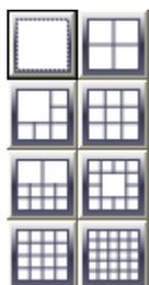
DX-PC200 has basic layouts. When the Existing grouping button under the User grouping buttons is clicked, the Basic Layout icons appear. When you select a layout, the screen layout changes accordingly.
