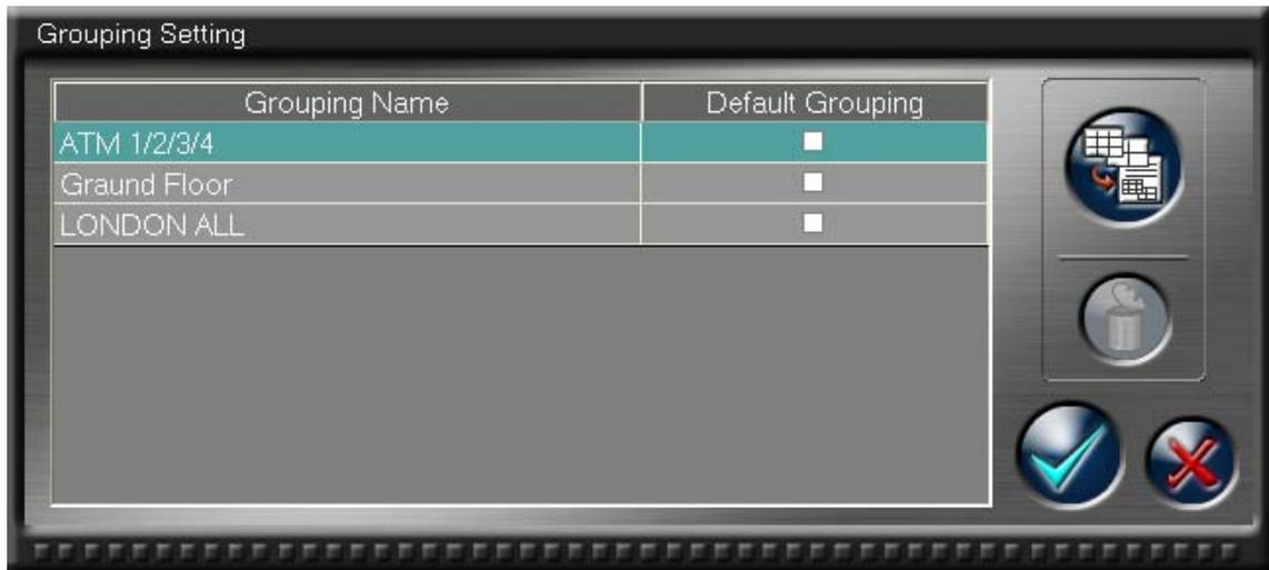
You can add or delete a grouping using the Regist button or the Deletion button located at the right section of this panel.
