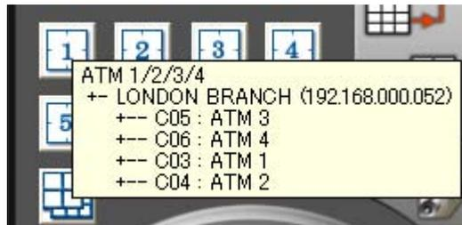
When you want to allocate a new grouping to a button to which a grouping has already been allocated, right-click the button. When the Grouping Select dialog appears, you can select a grouping.
