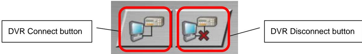
When the DVR Connect button is clicked, DX-PC200 shows the list of the disconnected recorders.
