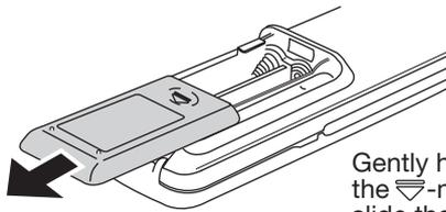
Gently holding down the
