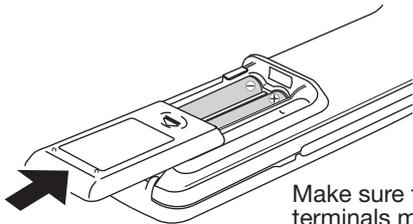
Make sure that the terminals match the  $\oplus$  and  $\ominus$  indications in the battery compartment.
