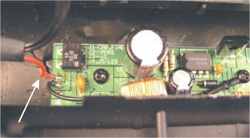
Locate the engine's constant voltage board power pickup wire as shown.
