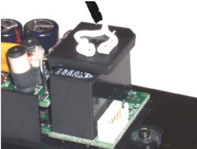
Apply white thermally conductive grease to bridge rectifier & metal heat sink bracket.
