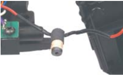
Install the inductor between the engine's power pickup lead and the power lead going to the constant voltage board.
