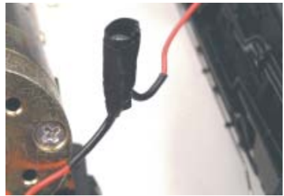
After soldering the inductor into place, use shrink tubing and electrical tape to insulate the inductor completely.
