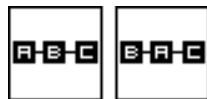
Figure 32: The four topologies in which the effects can be applied after the Amp module of the two module rows; A = Chorus module, B = Delay module and C = Reverb module.
