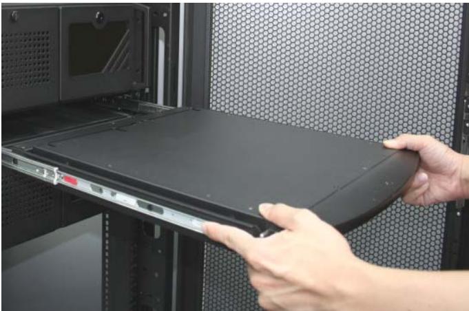
Figure 8. Pushing the white arrow button.
