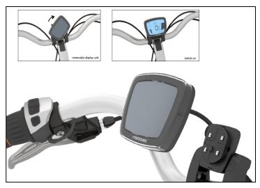
system. In other words the display also functions as a key to the electrical system. After the display is inserted turn on the battery. If the display is not mounted on the e-bike, the e-bike will works like a conventional bike.
