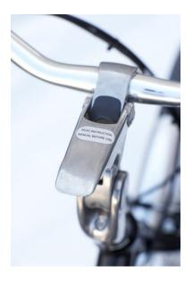
Push up the black button and raise the lever to allow for adjustment of the handlebars in desired position.
