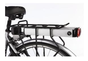
Turn the battery key (ON/OFF) to open position and take the battery out of the rack.
