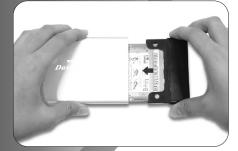
Slide in the HDD into the case
