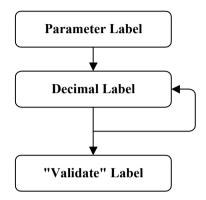
For example, to configure the Inter-Character Delay to be 15 ms, the "Inter-Character Delay" label is first read, and then the decimal digit labels "1" and "5", and finally, the "Validate" label to complete the setting.
