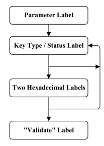
For example, to configure the Prefix Code to be "AB", the "Prefix Code" label is first read, and then the hexadecimal digit labels "4", "1", "4", and "2" are read, and finally, the "Validate" label to complete the setting.
