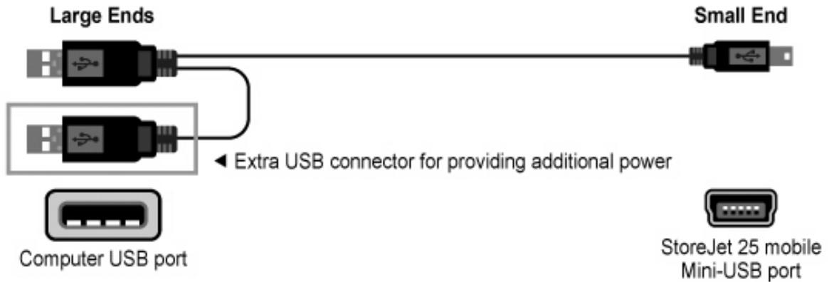
Figure 3: Mini USB to Standard-A USB cable (USB Y-cable)
