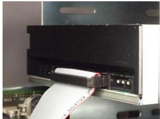
**Figure 3. Installing BUS Cable**
