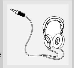
Once headphones are connected, "HEADPHONE DOWN MIX 2 CHANNEL" will scroll on display. This feature automatically converts multi-channel speaker outputs to 2 channel stereo for your listening pleasure.
