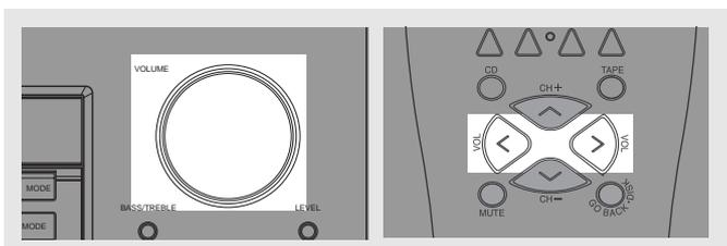
3. To adjust individual speaker volume level, press the **LEVEL** key on the main unit when the short noise is played on the speaker you want to adjust then turn the **VOLUME** knob to modify the output level.
