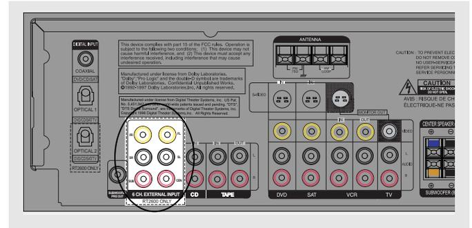
To activate 6 Channel external input, press the source key on the receiver until 6 CH is selected or press **DVD/6 CH** twice on the remote control.
