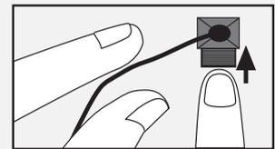
Release tab to lock wire in the terminal.
