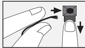
Push terminal tab down to insert wire.
