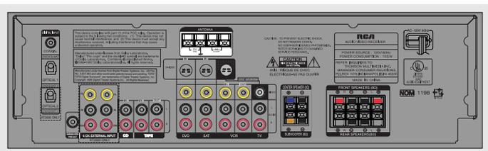
The AM and FM antennas connect to the AM and FM terminals on the system's back panel.
