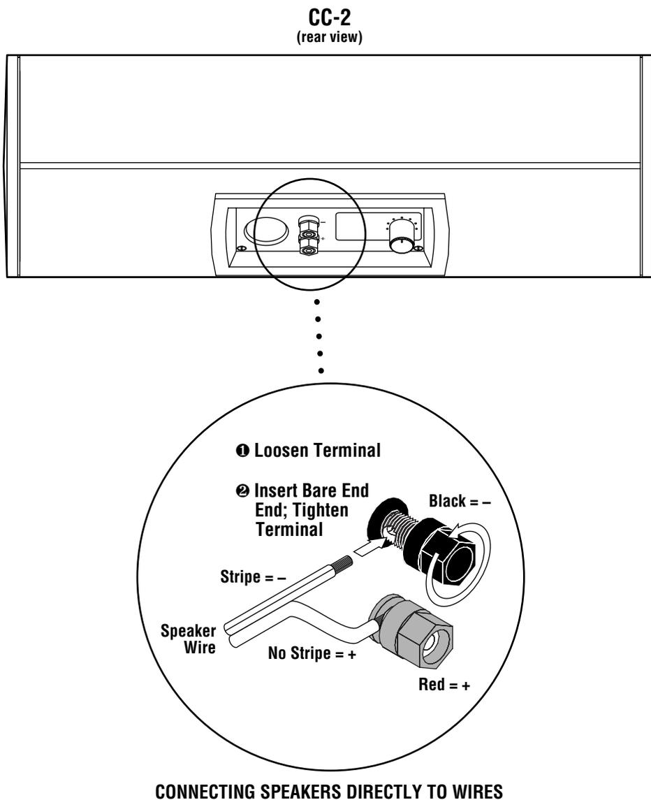
Figure 5. This wiring diagram shows polarity connections for a center channel connection (also see the owner's manual that came with your amplifier, receiver, or television).
