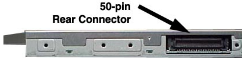
Figure 1. SD-R2412 DVD Writeable Drive Rear Panel – Connector
