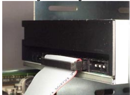
Figure 3. Installing BUS Cable
