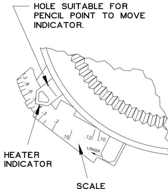
**Figure 5: Heat Anticipator Adjustment Scale**
