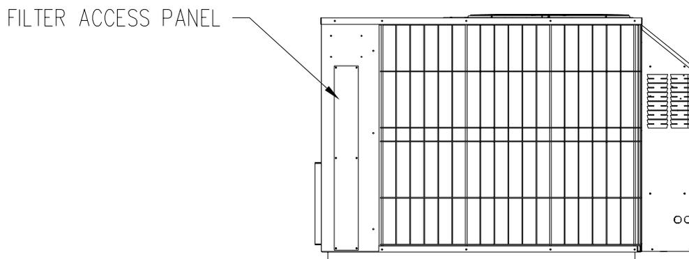
**Figure 12: Location of the OPB Supply/Return Air Filter**
