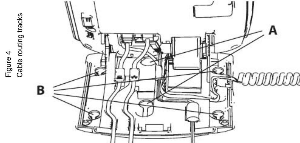
**Step 8: Wall-mount your phone (optional).** Your IPPhone1140E can be mounted either by: (Method A) using the mounting holes on the bottom of the phone stand, or (Method B) using a traditional style wall-mount box with RJ-45 connector and 15-cm (6-inch) CAT5e cable (not provided).
