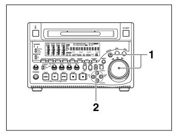
1 Hold down the SHUTTLE button, and turn the jog dial or shuttle dial.
