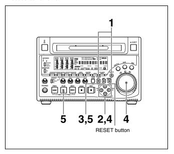
Hold down the SHIFT button, and press the THUMBNAIL button, turning it on.
