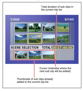
To move the cursor in the scene selection window After carrying out step **3** to display the scene selection window, press the  $\Leftrightarrow$  or  $\Rightarrow$  button.
