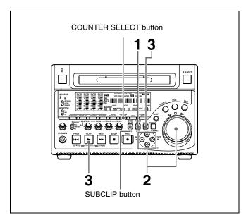
1 With the SUBCLIP button off, press the THUMBNAIL button, turning it on.
