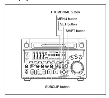
With the THUMBNAIL button off, hold down the SHIFT button and press the SUBCLIP button.
