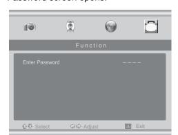
4 Enter the password with the number buttons on the remote control (the default password is 0000). The Parental Control sub-menu opens.
