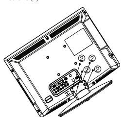
6 Reattach the shield panel with the ST3 screws (1) you previously removed.
