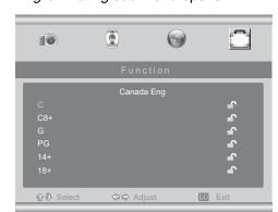
6 Press ▲/▼ to select the TV rating you want, then press ◀/▶ or ENTER to block or unblock the rating. The lock icon (♠) indicates the level is blocked, the unlocked icon (♠) indicates the level is unblocked.
