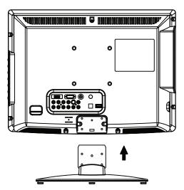
**5** Secure the pedestal stand with four M4 screws (2).
