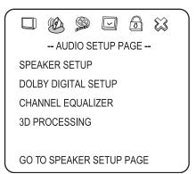
3 Press ▲ / ▼ to highlight 3D PROCESSING, then press ENTER. The 3D Processing Page opens.
