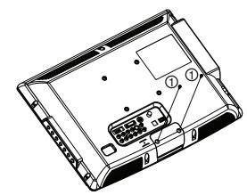
3 Remove the shield panel from the bottom of the back of the TV.
