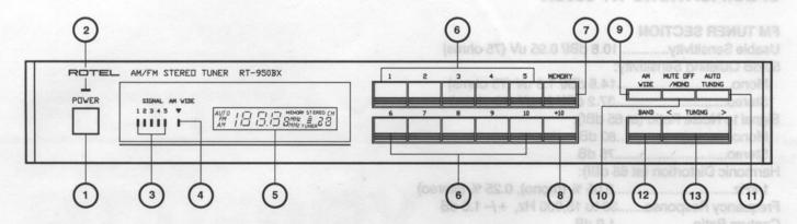
that the wide position is selected. If there is too much hiss or noise from neighboring stations, etc., press the Button to deactivate the Wide circuit and back to the normal bandwidth position for reducing such noise to negligible.
