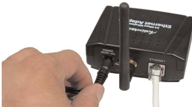
5. Plug the other end of the Power Cord into an power outlet.
