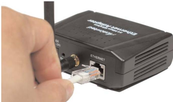
3. Plug the other end of the Yellow cable into the Ethernet port located on the back of the Computer or Game Console (like a Sony Playstation or Xbox). You will hear a “click” when the Yellow Cable has been properly connected.
