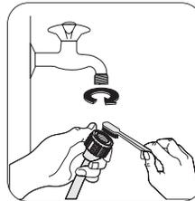
Turn off the water tap. Unscrew the water inlet hose. Clean the filter using a hard bristle brush. Refit the inlet hose.
