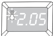
During the washing cycle the display shows a temperature icon to indicate that the appliance has started the heating phase of the water in the tub.
