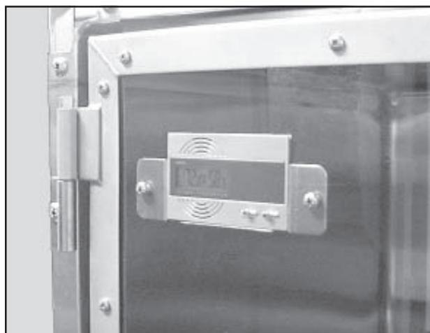
Figure 11. Temperature/Humidity Gauge
