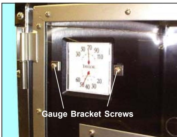
Figure 22. Removing the Old-style Gauge Assembly
