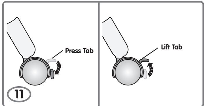
**To Lock:** Press the tab on all four wheels down until you hear a “snap”.
