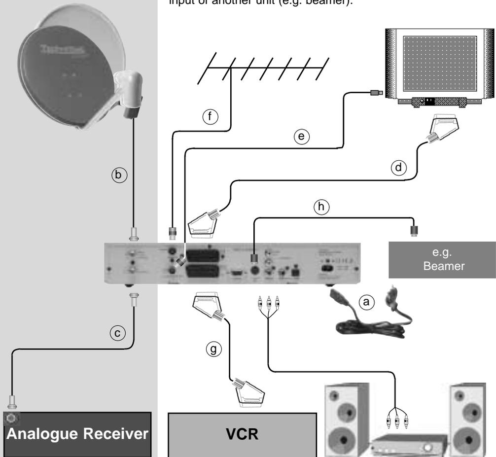
television set (SCART socket) by means of a SCART
