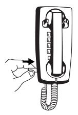
1. Slide out the lock lever 2. Place the keyhole slots over the wall mount plate's studs as you plug the phone's connector into the jack. Then slide down the phone to secure it.
