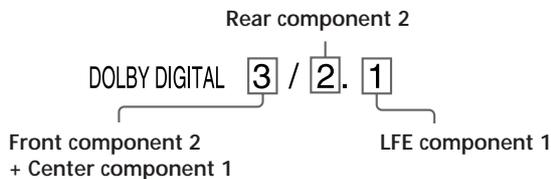
\*\* The playing channel shows the signals from 5.1 OUTPUT connectors whether the speakers exist or not. The letters in the channel display mean the following:
