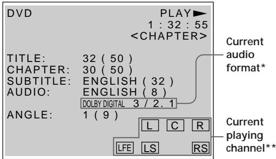
\* "PCM", "MPEG" or "DOLBY DIGITAL" is displayed. In "DOLBY DIGITAL" case, the channels in the playing track are displayed by number as follows:
