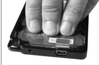
8. Connect the CE IDE (zif) cable to the drive, such that the label of the hard drive is facing upward\*\*\*.
