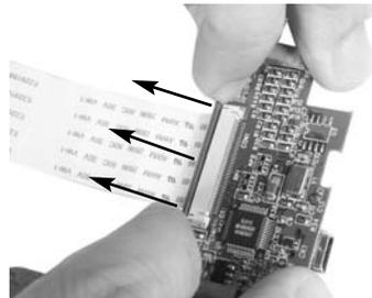
*Insert the Hitachi ZIF cable into the slot, ensuring the blue tab is facing upward, in relation to the ZIF connector. Once the cable has been firmly placed, gently press the tab (brown) back in place, in order to secure the cable.*
