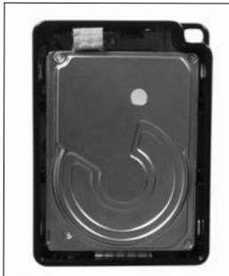
10. Place the front panel over the drive, by situating the bottom of the panel inside the enclosure, then securing the remainder:
