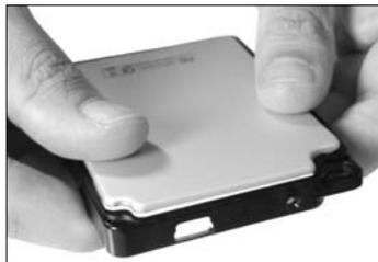
7. Insert the circuit board (removed in step #3) into the enclosure by aligning the USB connector (provided by the circuit board) with the USB port (provided by the frame), and gently applying pressure to the bottom of the circuit board until it is locked in place:
