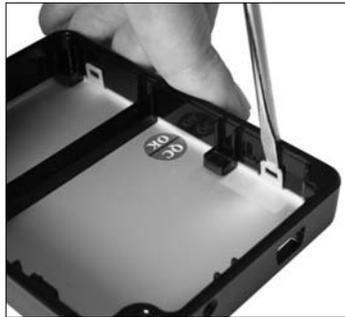
5. Once the clips have been loosened, remove the rear panel from the enclosure:
