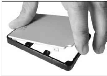
6. Fasten the rear panel (removed in step 5) to the alternately-sized enclosure frame:
