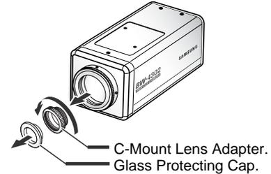
2. Attach the lens into the camera by turning clockwise.
