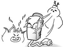
Do use the camera under conditions where temperatures are within -10 C to 50 C. Especially be careful for ventilation under high temperature.
