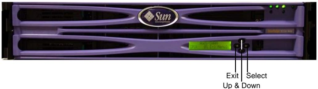
**FIGURE 2-5** The LCD Panel Controls
