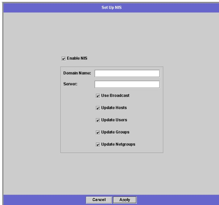
**FIGURE 6-1** The Set Up NIS Panel
