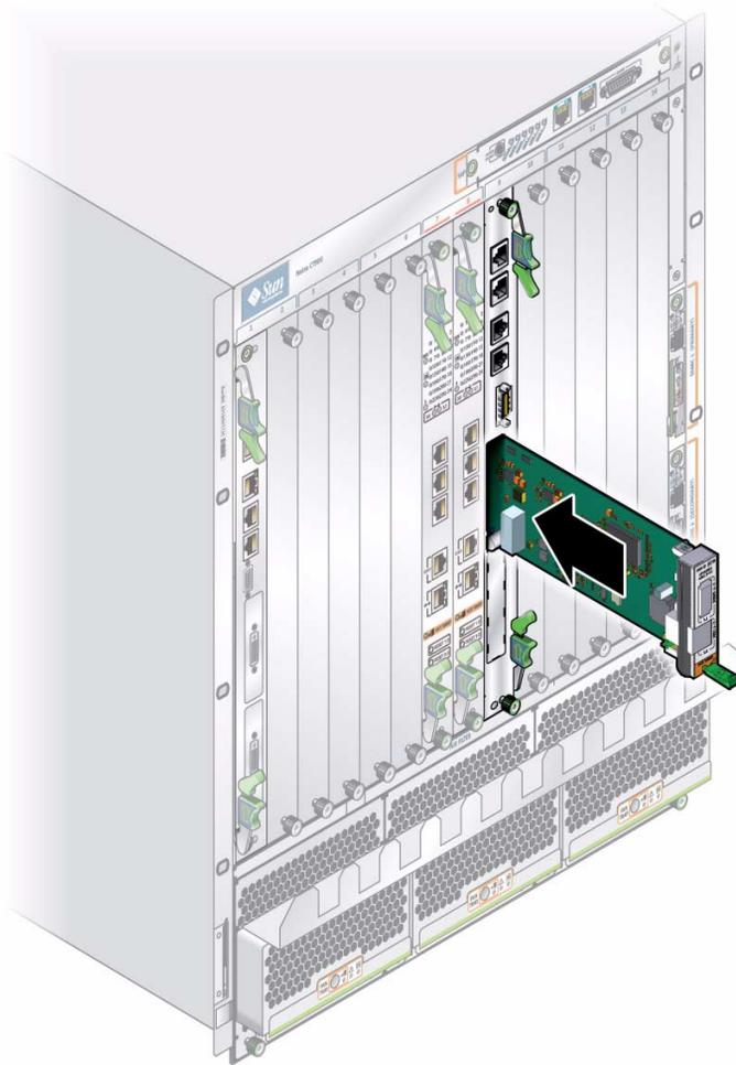
**8. Push the ejector latch in fully.**
