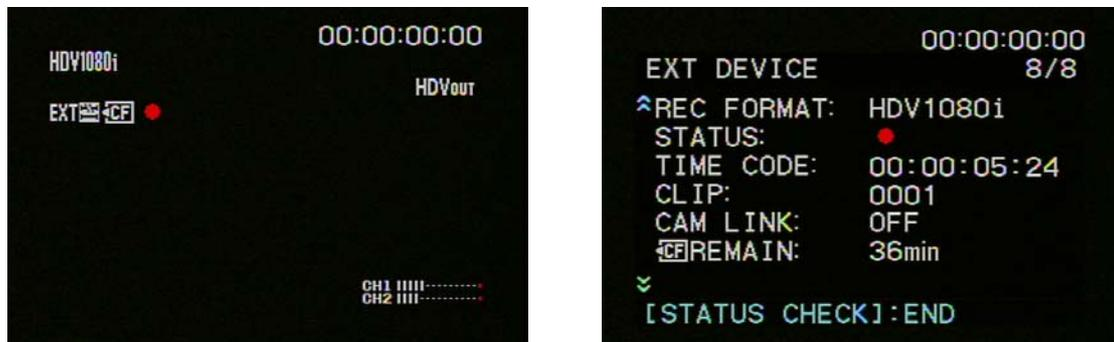
Figure 5. Screen shots from HVR-Z7E showing main screen on-screen display (left) and the additional page in the status menu (right)
