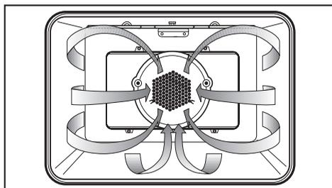
When using the convection function, several runner levels can be used at the same time.
