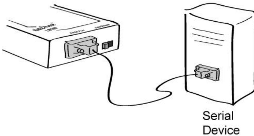
Figure 2-4. Connecting a serial device to the LS100
