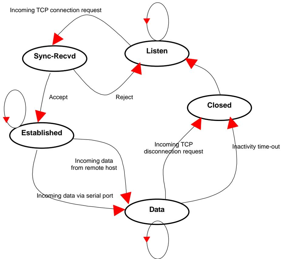
Figure 4-1. State Transition Diagram of TCP server mode
