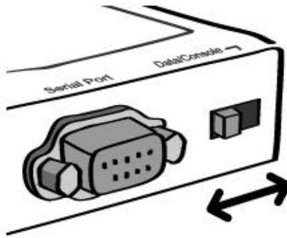
Figure 2-6. Data/Console switch of the LS100
