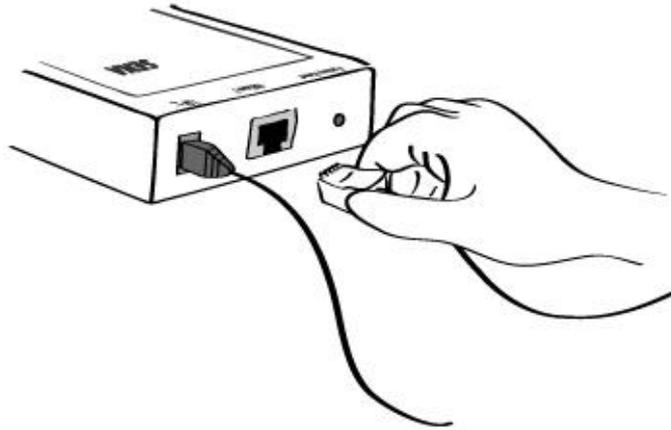
Figure 2-3. Connecting a network cable to the LS100
