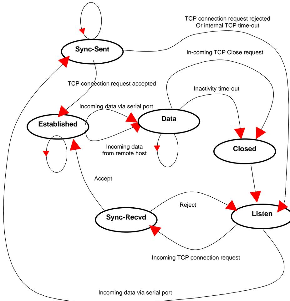
Figure 4-5. State Transition Diagram of TCP server/client mode
