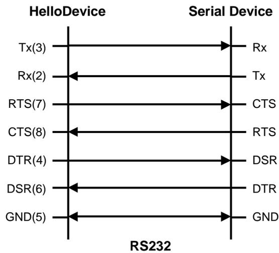
Figure A-5 RS232 wiring diagram
