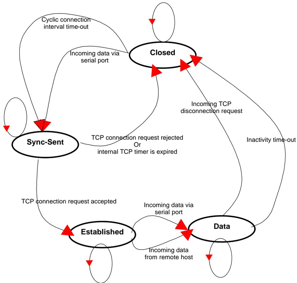
Figure 4-3. State Transition Diagram of TCP client mode
