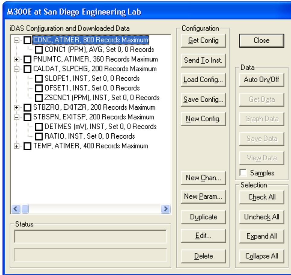
**Figure 4-1: iDAS Configuration and Downloaded Data Dialog**
