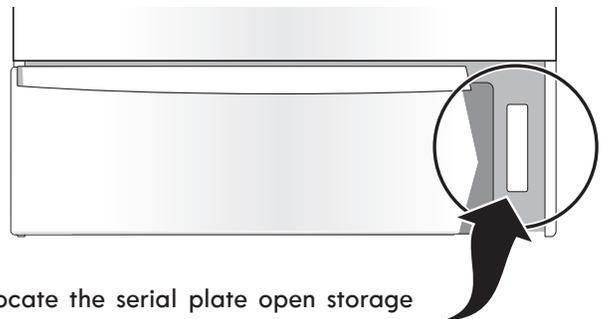
To locate the serial plate open storage drawer (some models) or warmer drawer (some models). The serial plate is attached to the lower right oven frame.
