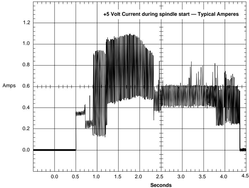
Figure 2. Typical 5V startup and operation current profile
