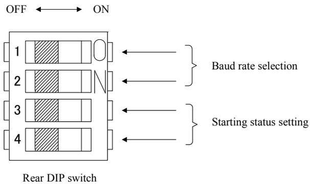
(1) Baud rate setting: Baud rate setting of camera IN /OUT
