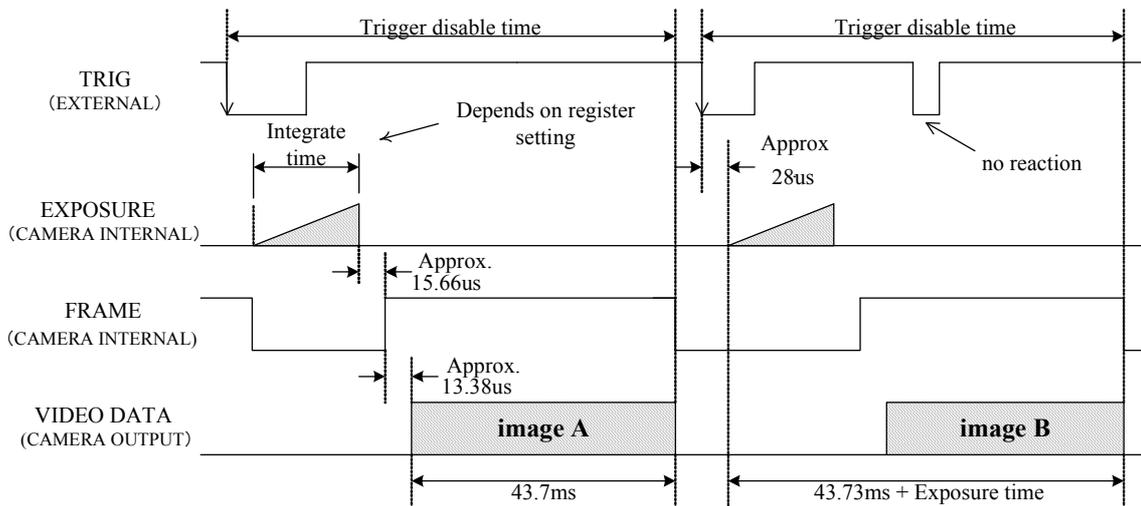
Shutter speed depends on the internal register setting value.
