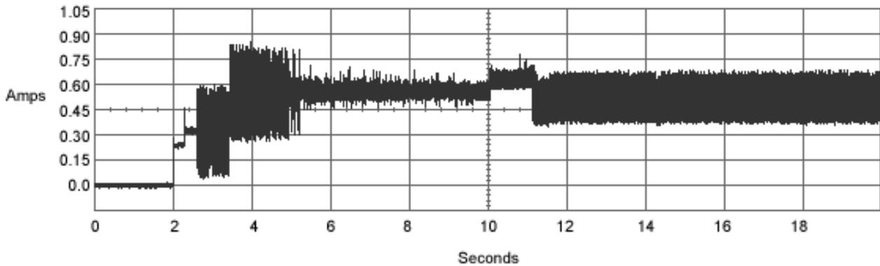
**Figure 1. Typical 5V startup and operation current profile**
