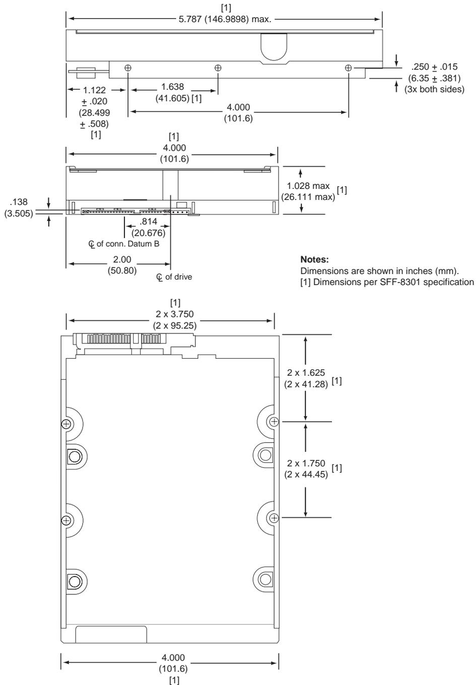
Figure 5. Mounting dimensions—top, side and end view
