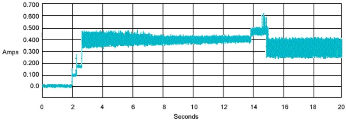
Figure 1 Typical 5V startup and operation current profile
