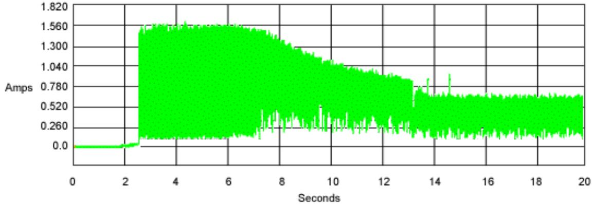
Figure 2 Typical 12V startup and operation current profile
