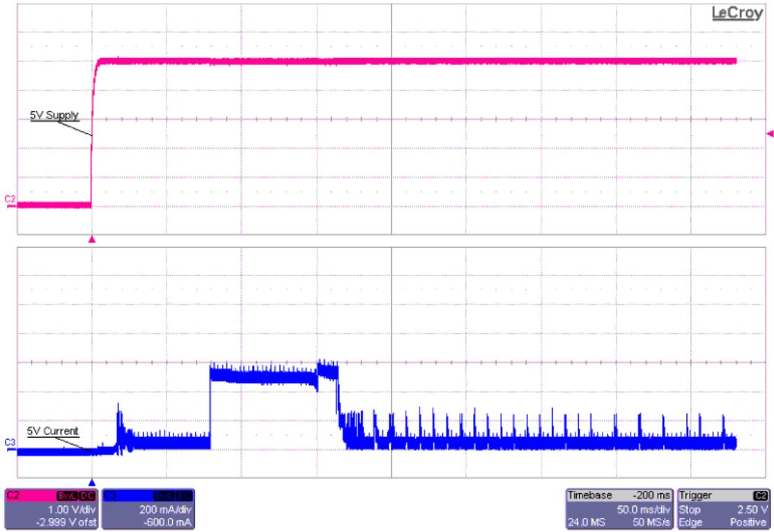
Figure 1. Typical 5V Startup and Operation Current Profile
