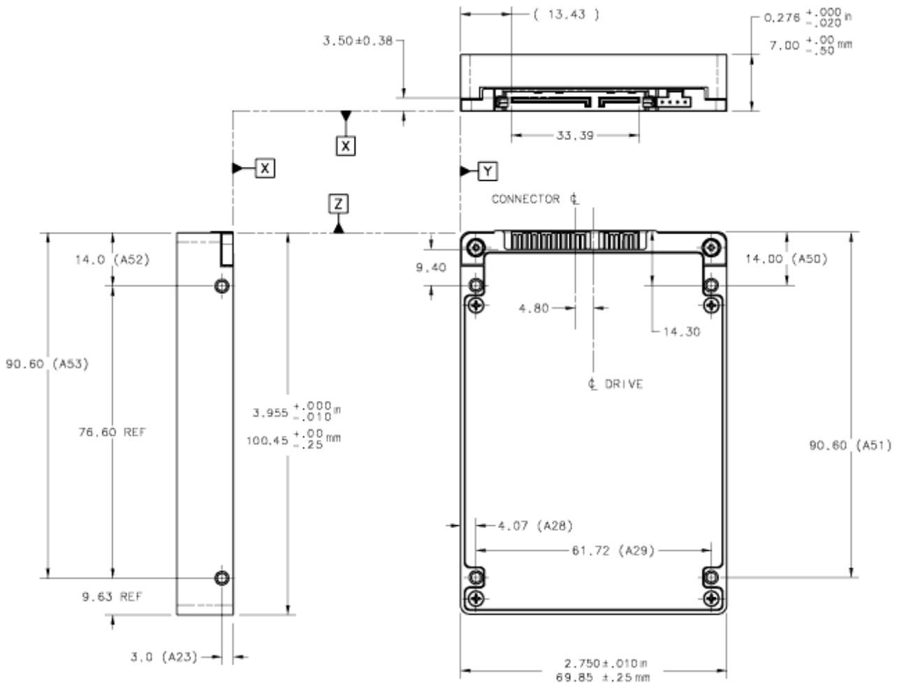
**Figure 3. Mounting configuration dimensions (7mm models)**
