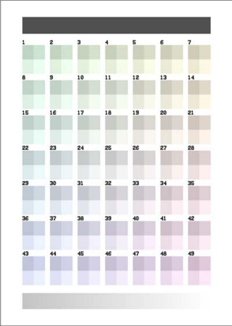
3. Examine the test print from the printer to determine the most neutral gray patch. Then click the patch in the Calibration Utility screen that corresponds with the most neutral patch on the test print.
