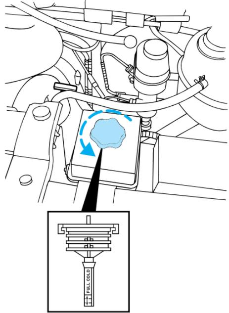
1. Start the engine and let it run until it reaches normal operating temperature (the engine coolant temperature gauge will be near the center of the NORMAL band).
