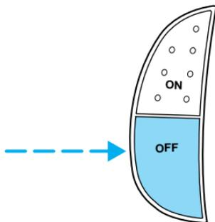
Once speed control is switched off, the previously programmed set speed will be erased.
