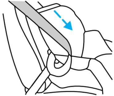
6. Allow the belt to retract. The belt will click as it retracts to indicate it is in the automatic locking mode.
