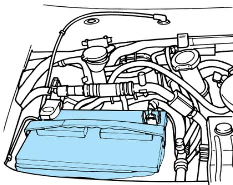
If the electrolyte level in the battery is low, you can add plain tap water to the battery, as long as you do not use hard water (water with a high alkali content). If possible, however, try to only fill the battery cells with distilled water. If the battery needs water often, have the charging system checked.
