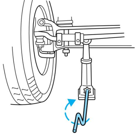
3. Turn the jack handle clockwise until the wheel is completely off the ground.
