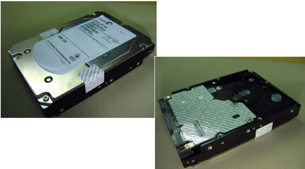
Figure 26. Example of FIPS tamper evidence labels.
